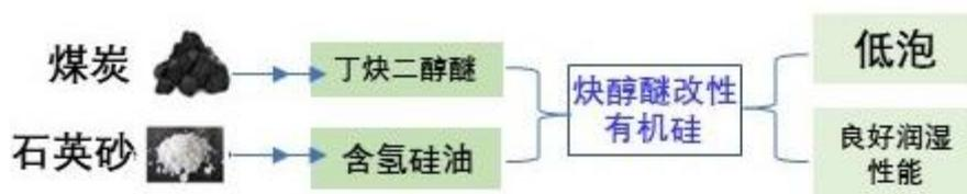
Fig.1 Schematic diagram of development of butynediol-ethoxylate siloxane
