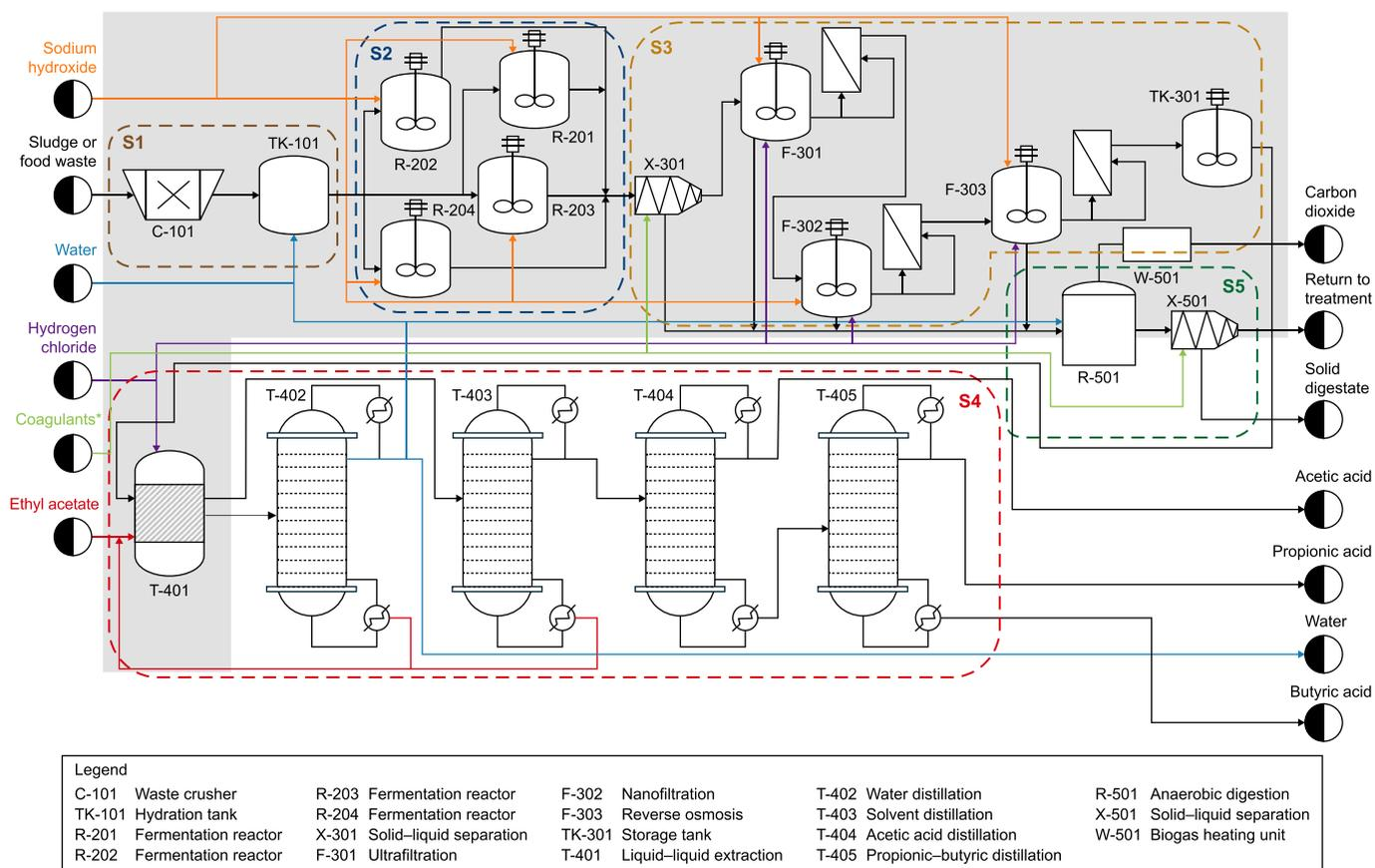
**Fig. 1.** Plug flow diagram of the sewage sludge or food waste biorefinery. The gray shading indicates the boundaries from which the pilot-scale primary data were collected. The color of the arrows is related to the chemical fed to each equipment. S1: Pretreatment and water addition; S2: Fermentation; S3: Solid-liquid separation and VFAs pre-concentration; S4: VFAs purification; S5: Solid fraction digestion.
