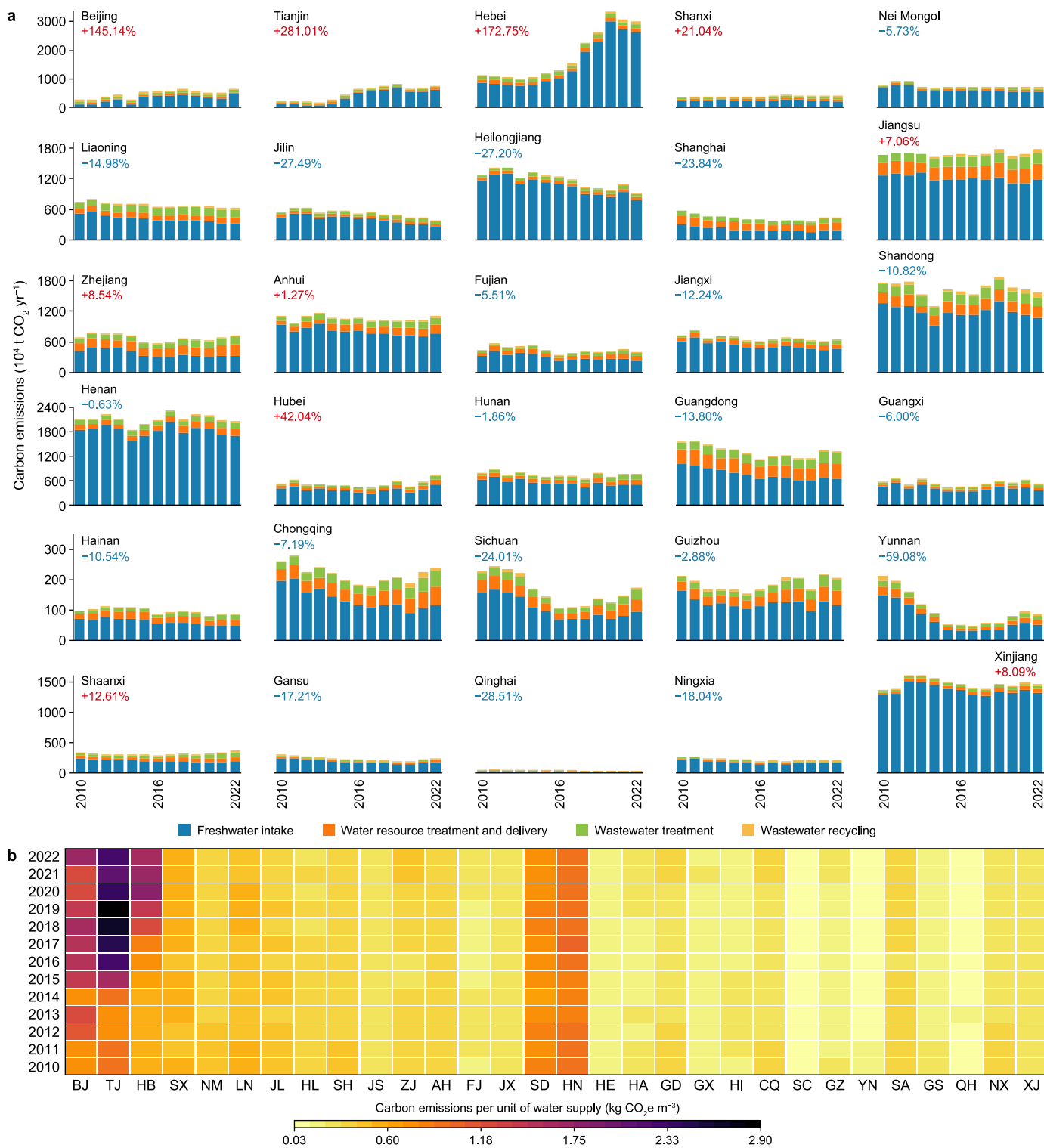
Fig. 3. Provincial trends in carbon emissions from water-supply processes (2010–2022). a , Carbon emissions by water-supply stage for each province over time. The red and blue numbers represent changing rates in carbon emissions in 2022 relative to 2010. b , Carbon emissions per unit of water supplied for each province over time.
